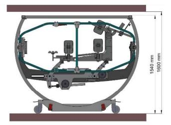
Figure 3: Height in folded configuration
